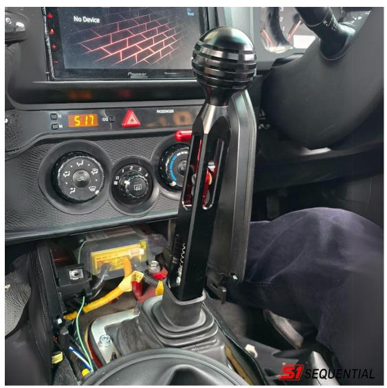
17. Refit trims and fit the shift knob with the supplied M12 stud and some Loctite and the project is complete, If you want to run a different shift knob look for something with an M12x1.75mm thread
