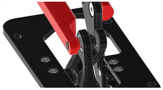
6. Attach the support rod to the shifter with the M8x30 button head bolt. And place supplied rubber bushes in the front of the support rod.
