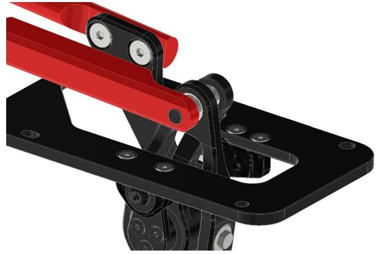
4. Assemble shift rod, the center the center measurement should be about 225mm but this can be adjusted late to suit your preference. The M6x20 bolts should be placed in but not tightened.
