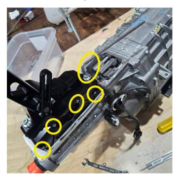
**30.** Fit front left bolt M6x20 ( the washer for this only has a 6mm hole not an 8 like the others) and also fit rear left bolt (M8x35 socket cap head bolt).
