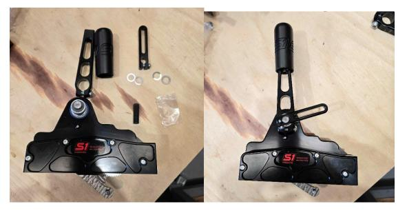
Make sure you play with the shifter a bit before fitting so you understand how it works and keep in mind that the shifts will feel quite stiff when the shifter is not fitted to the box do to the indexing mechanism. I would recommend placing the front of rear edge of the shifter on a bench when trying to shift it so you can apply enough force, you will not be able to change gears just holding the shifter in your hands.
