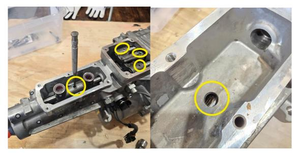
**3.** Remove parts circled, make sure to remove the neutral switch extender from the housing.
