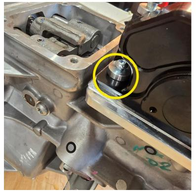
**31.** Give it all one final test and everything is good fit the drill square part to the rear of the shifter using the M5x30 countersunk and the M5x25 socket head cap screw making
