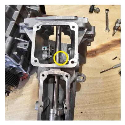
**12.** Check for clearance when rotating shaft and fitting, on the right side it should be able to turn until the flat of the shaft fitting is parallel with the cut section of the case.
