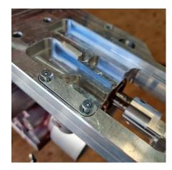
9. Fit the reverse lock out lever, this can be set at any angle that suits you.
