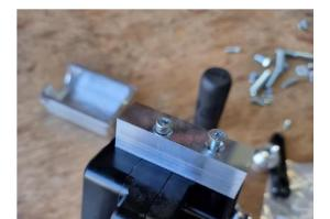
17. Drill 6mm holes for the roll pins through the drill square part and the base plate. Once fitted these will stop the shifter from moving under high driving loads. THESE MUST BE FITTED do not try an alternative method this is the correct one.
