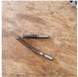
5. Remove centering plunger and fit the supplied aluminum spacers underneath, these will apply a rotational force to keep the shifter at the 1<sup>st</sup> or reverse side of the gate when needed
