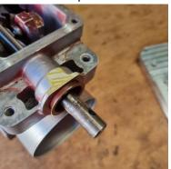
7. Fit shaft fitting using original roll pins.
