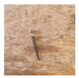
4. Remove both left and right side plungers and refit cover using a 27mm socket.
