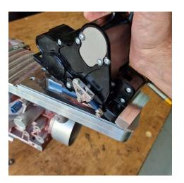
15. Bolt down the shifter with the aluminium washes fitted so it will still be free to move a bit of not centred perfectly. Shift though the gears to check operation. Once everything is working mark the shifter position with a scribe to make any refitment easier.
