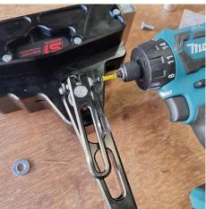
10. Fit the shift knob. 2x M12x1.75mm studs are provided the long one should be wound into the shift knob (there is a socket in one end) the shorter one is used if you choose to use the spacer for might lever height or leverage. The shims provided are so you can align the shift pattern.
