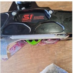
Once the cam is in the position between first and second gears the reverse lock out lever should be free to move which will also move the side shift arm that is the steel part under the shifter with the ball like fitting on the end.
