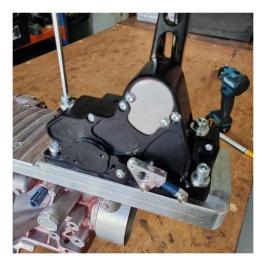
16. Fit the drill square part the rear of the shifter. Using the socket and countersunk M5 screws.
