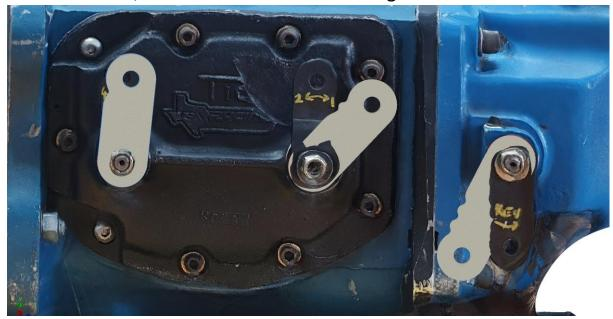
4. Use the m10x25 countersunk bolts to attach the shift lever and reverse lock out lever.
