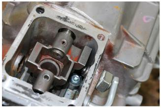
on these gearboxes this ball plunger must be removed and replaced with the provided bung.
