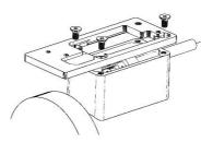
5. Fit base spacer with a thin layer of sealant.
