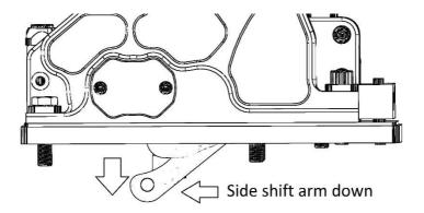
12. Slide the ball shaped fitting on the side shift arm into the groove on the left side of the shaft fitting as you lower the shifter onto the base plate. Check that the shifter slides all the way flush with the base, do not force it down with bolts.
