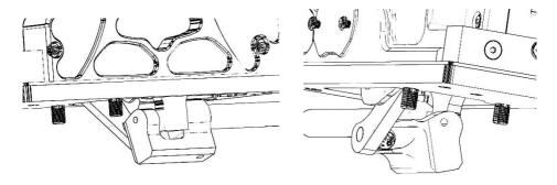
13. Fit and slightly tighten the three 8mm cap head bolts to attach the shifter to base plate then rotate the reverse selector back and forth a few times to get a feel of it.
